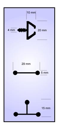
Rigid P.V.C. screen edge profiles combined with flexible dumbell sections.
