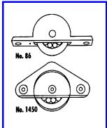
The No.86 Bottom Track is steel bonderised and epoxy coated to resist rust. Wheel units with steel ball bearings for free running encased in a glass reinforced nylon tyre for strength and effortless movement.
