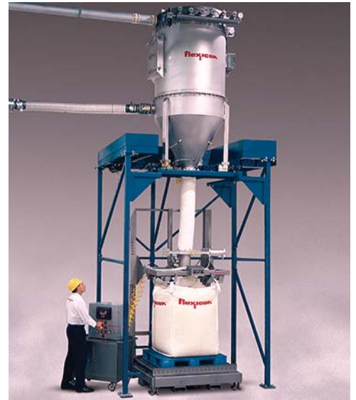
The filter receiver's load cells transmit weight gain information to the system controller that stops the conveyor once a pre-selected batch weight, equivalent to that of one full bulk bag, has been accumulated.
