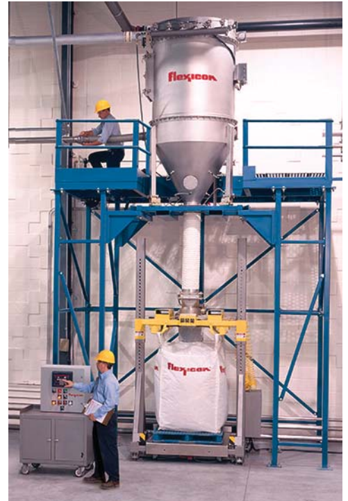
A PNEUMATI-CON® pneumatic conveying system weighs material and discharges it into a TWIN-CENTERPOST™ bulk bag filler at high rates, dust-free.
