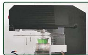
Stable granite stone machine structure
