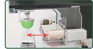
Pad in/out stroke for max. throat depth
