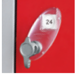
The Hasp & Staple allows padlock fitting. Shank diameter: min 6mm, max 7mm (Padlock sold separately).
