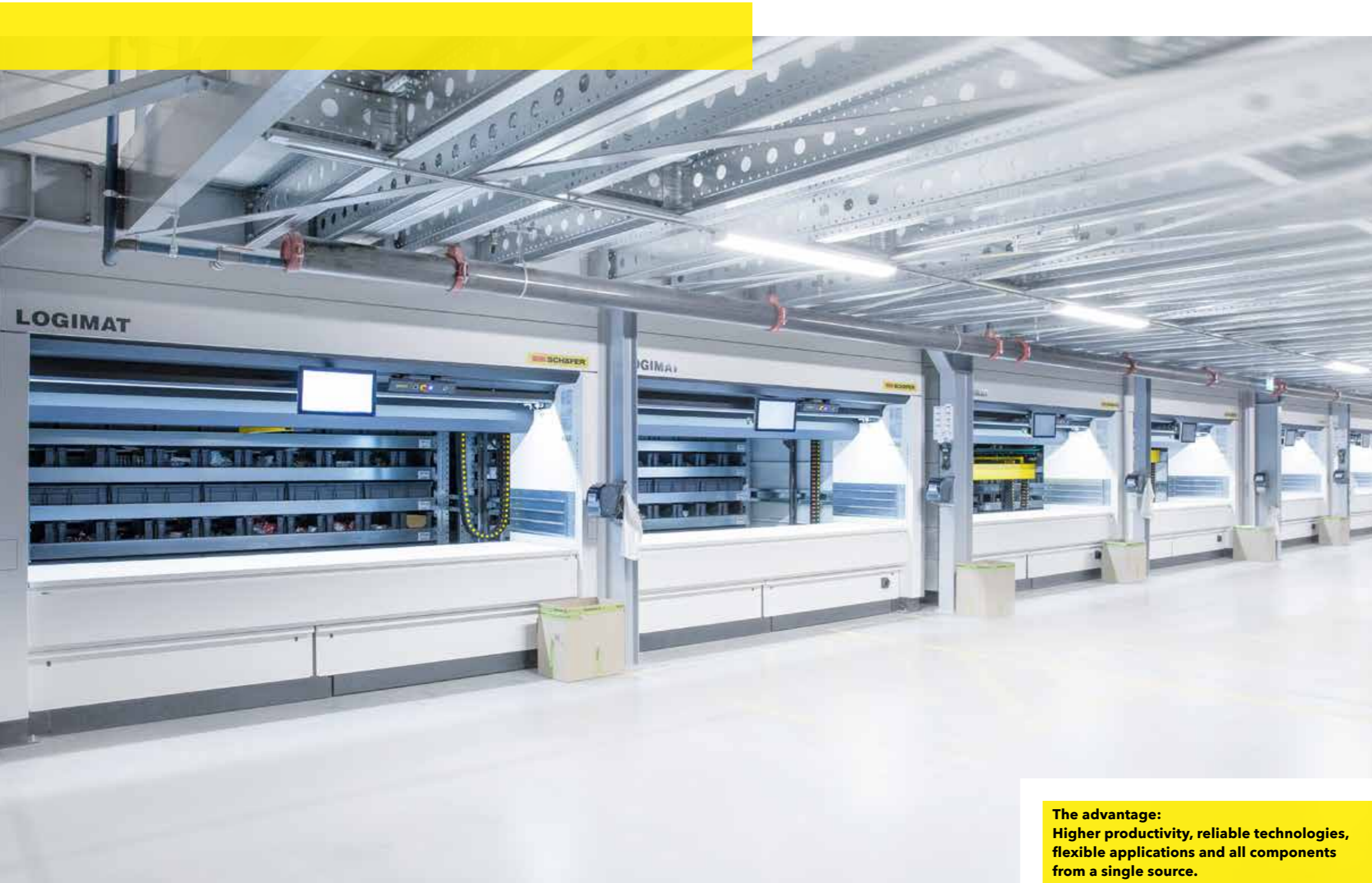
The Vertical Lift Module's operating opening is located on the „main level“ of the warehouse, allowing the Vertical Lift Module itself to be built from the basement up to the ceiling.
