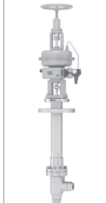
Type 3248-1 Cryogenic Valve, aluminum angle valve with positioner, supply pressure regulator, pressure gauges and additional handwheel
