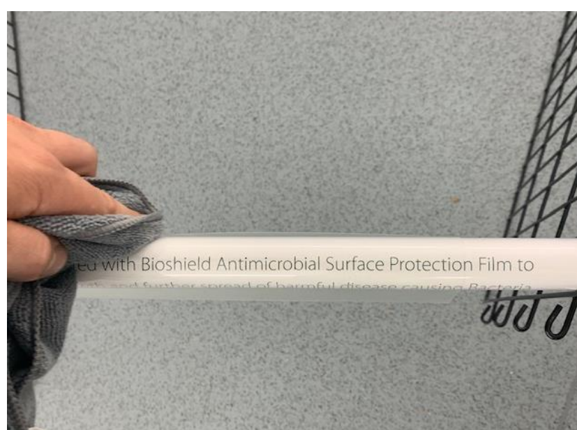
Step 5 – Work your way around the top of the handle, firmly pushing the kit down to push out any air.
