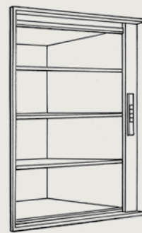
One or more shelves heating food and crockery from the bottom up (maximum of four shelves).
