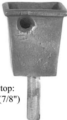
Internal measurement at top: 23mm (29/32") x 22mm (7/8")
