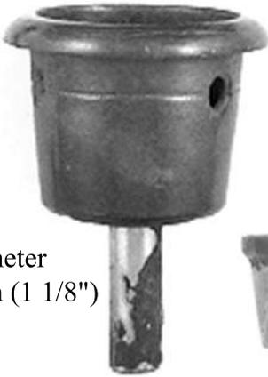
Internal diameter at top: 29mm (1 1/8")
