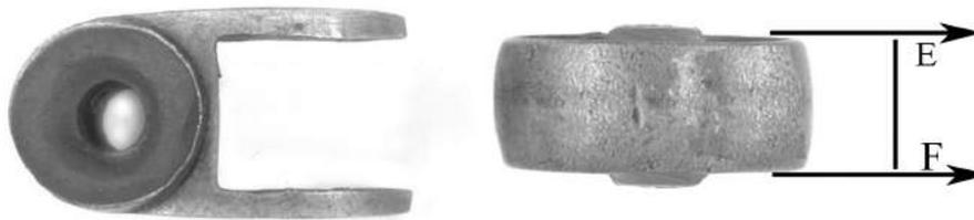
C - D Wheel diameters have been measured on the crown of the wheel.
