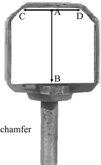
The A-B measurement= Maximum internal height
