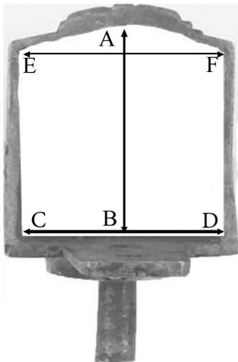
The A-B measurement= Maximum internal height
