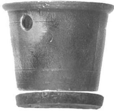
(Steel disc assembled at base of cup)
