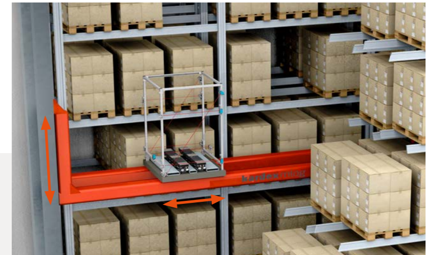
Via the lifting beam, the distribution vehicle services the pallet locations on the different levels.
