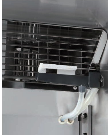
Wick inside chamber
