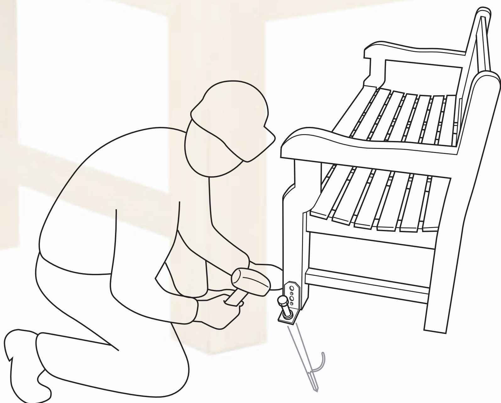
Drive the anchor into the ground
