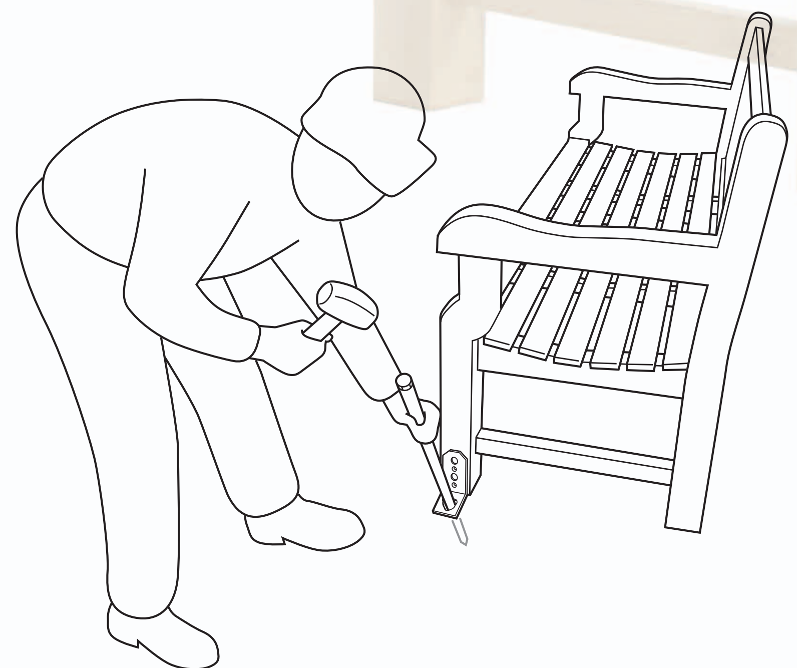
Drive out the fluke mechanism
