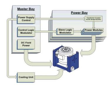
High performance MPA3000 Series amplifier has full power output of up to 300 kVA. Designed for use with ETS Solutions 'H' Series water cooled shakers and configurable to couple with any large sized water cooled shaker system. The power supply for the field coil, cooling unit, hydraulic unit or other ancillary units are provided by the amplifier. Integrated ancillary units can be part of the start-up and stop sequences.
