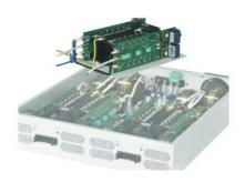
Designed with the latest high-advanced MOSFEF power transistors, the 12 kVA power unit consists of two self-regulating sub 6 kVA units.
