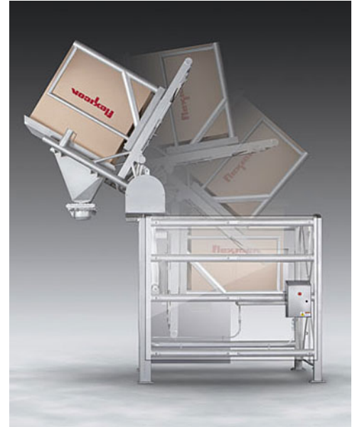
TIP-TITE® Sanitary Box Dumper forms a gasketted, dust-tight connection between the container and the equipment, tips the container to 45, 60, or 90 degrees past horizontal, and discharges bulk material through a slide gate at controlled rates.
