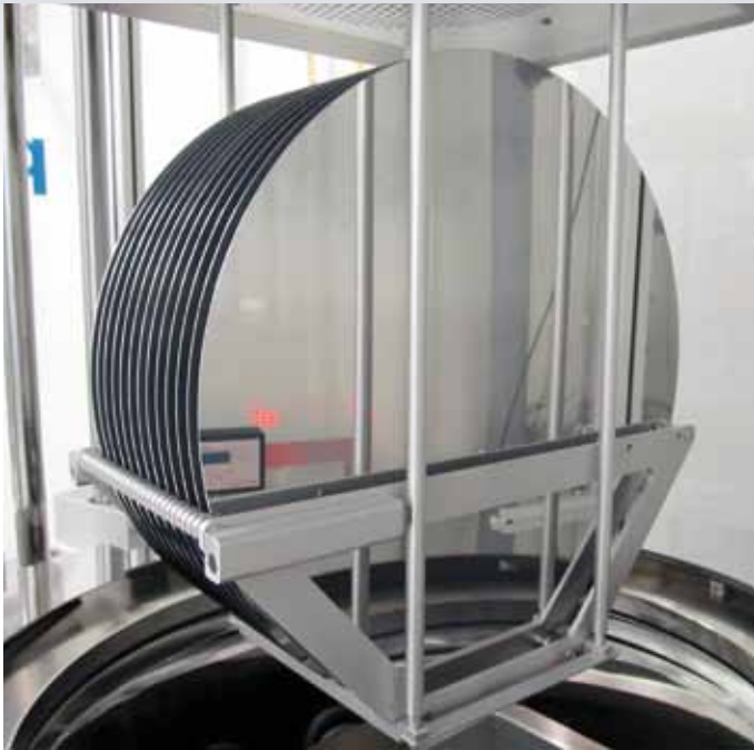
300 mm wafers coated in a PICOSUN™ P-300 batch reactor.
