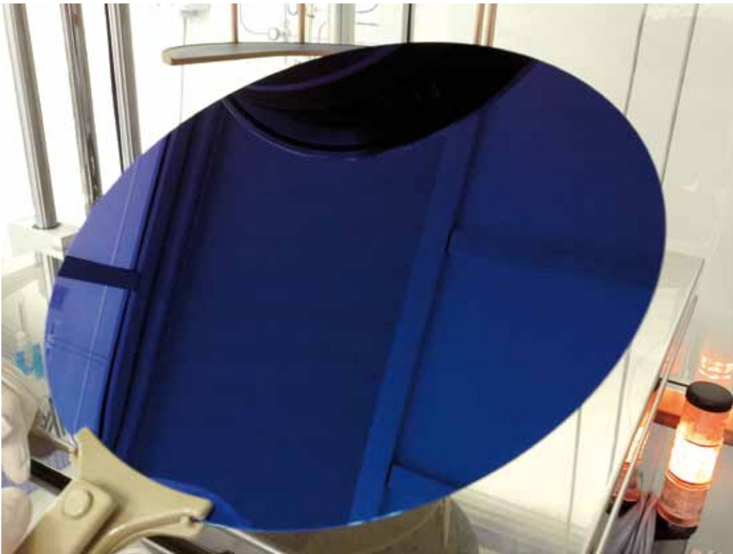
A 300 mm wafer coated in a P-300 single wafer reactor.
