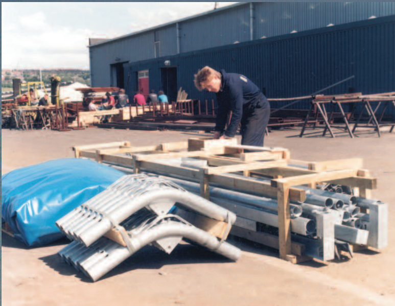
THA shelter components pack compactly for shipment.
