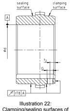
Clamping/sealing surfaces of types: FB, FAB and FH
