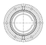
Illustration 30: Removing the locking screws and sealing washers
