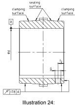
Clamping/sealing surfaces of types: DB, DAB and DH
