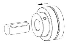
Illustration 31: Assembly of component assembly
