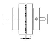
Illustration 19: Assembly of coupling
