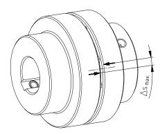
Illustration 38: Inspection of the limit of wear
