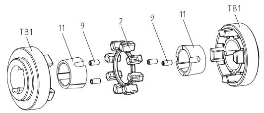
Illustration 15: POLY-NORM® type with taper clamping sleeve
