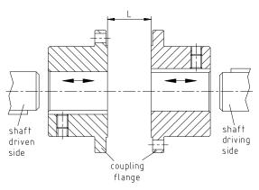
Illustration 26: Assembly of coupling flanges
