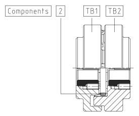
Illustration 16: Type with taper clamping sleeve hub design TB1 and TB2
