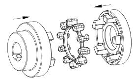
Illustration 30: Assembly of hub, elastomer ring and driving flange
