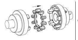
Illustration 18.1: Assembly of elastomer ring
