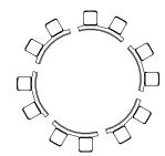
Illustration 24: Mounting aid of elastomer ring from size 75
