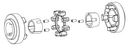
Illustration 33: POLY-NORM® type with taper clamping sleeve
