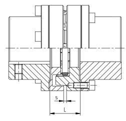
Illustration 28: Assembly of coupling
