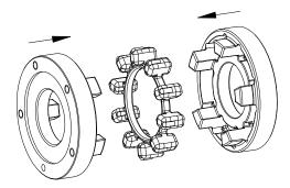
Illustration 27: Assembly of driving flange with elastomer ring
