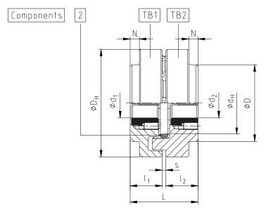
Illustration 8: POLY-NORM® type with taper clamping sleeve
