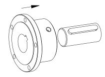
Illustration 29: Assembly of coupling flange
