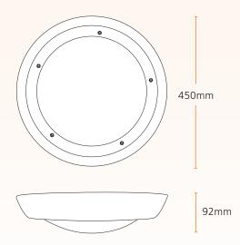
**AEGIS** is a 450mm diameter circular surface mounted luminaire of anti-ligature design suitable for areas where it is essential to prevent patient self harm. Supplied with tamper proof TP(a) rated low glare polycarbonate diffuser. Colour temperature 4000K. Available with anti-microbial paint finish. Anti-ligature when correctly installed using anti-pick mastic.
