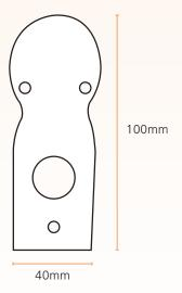
The **CM** range is designed to meet the strict hygiene requirements of many food production environments. The extruded aluminium tear drop profile with no dust traps or fins is rated IP65 to allow for wash down cleaning procedures.
