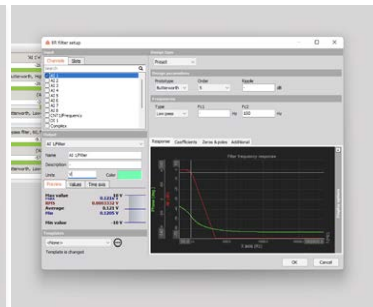
THE FILTER SETUP SCREEN FOR IIR FILTERS. FIR, CFC AND FREQUENCY DOMAIN FILTERS ARE ALSO AVAILABLE. YOUR RAW DATA IS NOT AFFECTED - A NEW CHANNEL IS CREATED.
