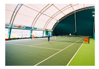
Features of the CopriSystems structure include a tensile membrane cover allowing natural light to flood the courts and hard-wearing material side walls which can be retracted during warmer months to allow for maximum ventilation.
