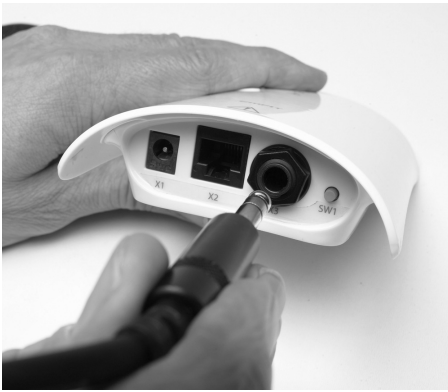
Connect the sensor wire plug to the control unit X3 marked connector.
