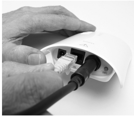
If you need to connect the dry-contact output to another system, plug the suitable connection wire to the X2 marked connector
