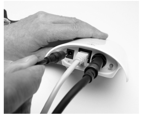
Connect the optional AC adapter cord to the X1 marked connector
