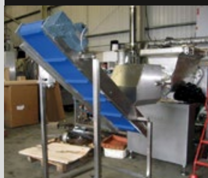
Incline flighted conveyor
