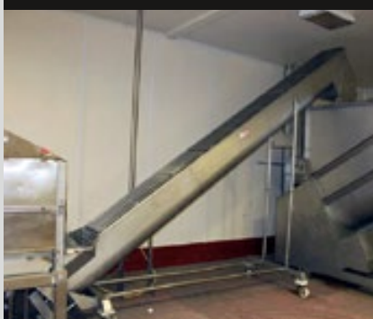
Boldt 400 mm incline screw auger
