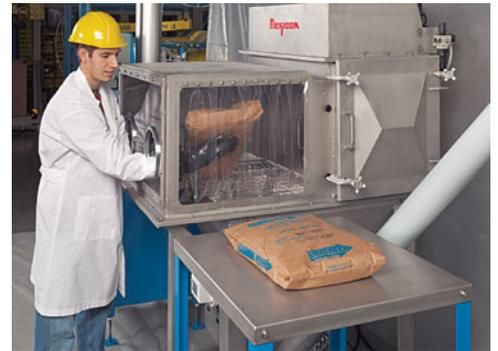
*The operator is isolated from dust by means of a dumping hood comprised of a plastic strip curtain, glove box, empty-bag infeed chute, and dust collector atop a receiving hopper feeding an enclosed flexible screw conveyor.*
