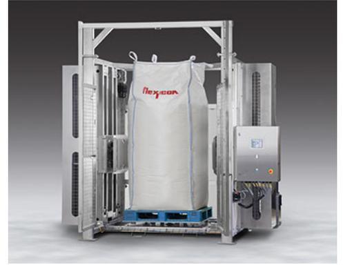
*This patented BLOCK-BUSTER® Bulk Bag Conditioner features hydraulically-actuated rams that automatically adjust in height for conditioning of short to extra-tall bulk bags, while reducing height of the loading deck by about 50 percent.*
