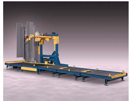
A 15-pallet dispenser releases the bottom-most pallet to roll beneath the cantilevered fill head of a bulk bag filler. Following manual connection of empty bags to the fill head, filling, densification and conveying functions are automatic.
