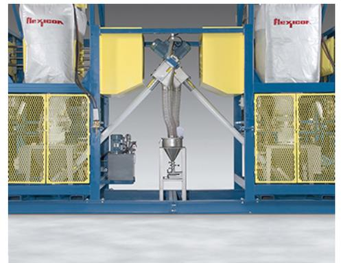
*Flexible screw conveyors gravimetrically feed bulk solids into a central solid-liquid eductor that blends the material into a liquid stream in ratios set by the user.*
