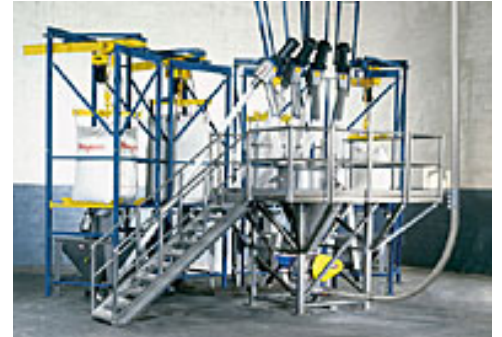
Feeds and weighs ingredients, and transports pre-weighed batches
