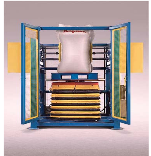
The combined action of a hydraulically- actuated, variable-height turntable, and two hydraulic rams with specially contoured conditioning plates, presses opposing sides of bulk bags at varying heights to loosen compacted materials.
