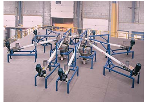
Automated low profile weigh batching system is comprised of eight low profile flexible screw conveyors fed by roof-mounted storage vessels, with each group of four conveyors feeding either of two gain-in-weight hoppers
