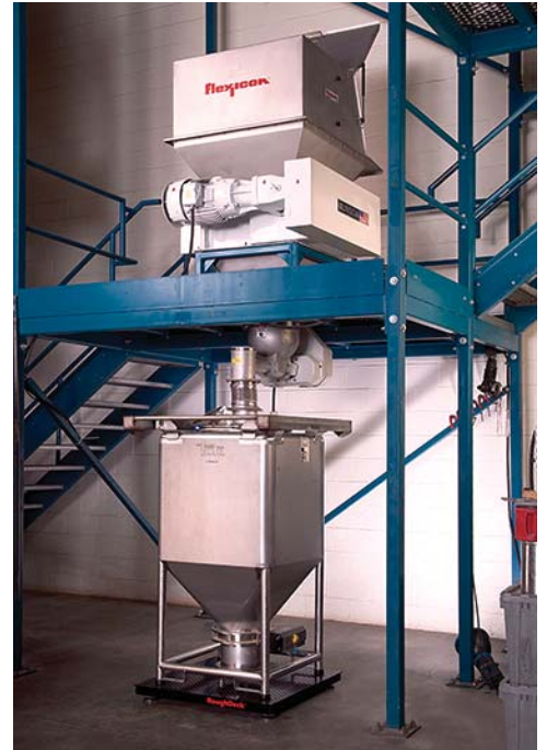
Manual Dump to Rigid Bin Weigh Batching System eliminates dust during manual dumping activities, de-lumps the material, and feeds it gravimetrically into rigid bins placed on a floor scale.
