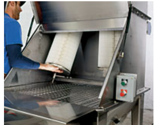
Timer activated solenoid valves release short blasts of air inside cartridge filters causing dust build-up to fall into the hopper. The hopper shown is configured for direct connection to a flexible screw conveyor. Other configurations allow connection to pneumatic conveyors or other conveyors and process equipment.
