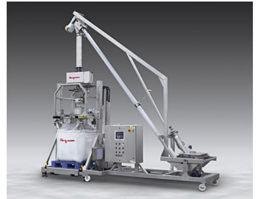
Mobile, Sanitary Bulk Bag Filling System from Flexicon is comprised of a TWIN-CENTERPOST™ Bulk Bag Filler with metal detection/removal, and a Tilt Down Flexible Screw Conveyor with clog-free dust-containment system. Programmable controls automate all filling and conveying functions.
