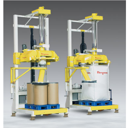
Combination bulk bag/drum filler features a fill head that pivots down to allow safe, rapid bag spout connections, and a swing-arm-mounted drum filling chute that automatically rotates to fill four drums on a pallet.
