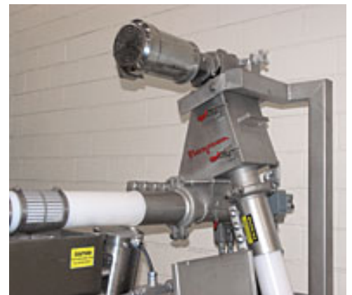
Flexicon Spreader-Feeder evenly distributes spices, seeds and other bulk coatings onto food products passing beneath the system's discharge hopper, while collecting and recirculating excess material.
