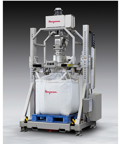
Sanitary, stainless steel TWIN-CENTERPOST™ Bulk Bag Filler with metal detection/removal weigh-fills and deaerates/densifies bulk bags, automatically and dust-free.
