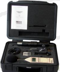
The measurement kit includes a tripod to allow the microphone to be positioned at the correct height along with an alignment tool to position the microphone at the correct angle to the exhaust.
