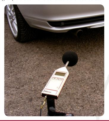
The CK:261S Measurement Kit includes a positioning template which can be used to ensure that the microphone capsule is set at the correct angle and distance from the vehicle exhaust.
