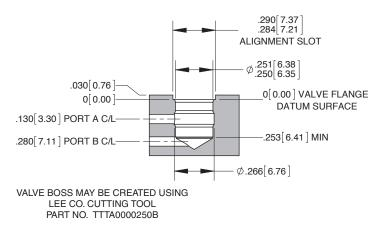
Reference Drawing Number LCFX0300250B for Plug-In Boss Detail.
