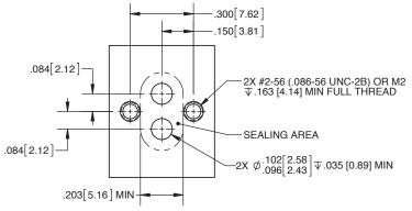
Reference Drawing Number LFIX1002050A for Face Mount Boss Detail.
