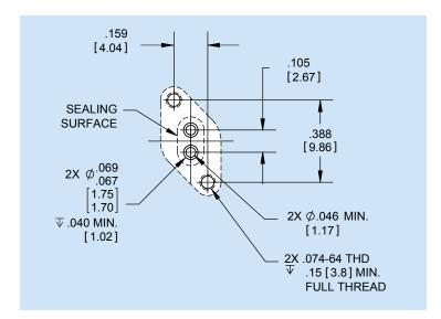
The LFNX boss is designed to simplify manifold construction. Manifold thickness is minimized, reducing fluid transport volumes and manifold material. (For full mounting boss details, use Lee drawing LSIX1001800A).
