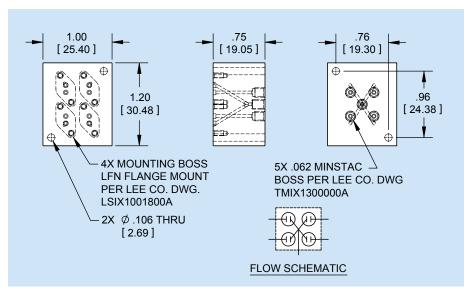
Lee 4 place manifolds (LSMX0512650B) allow 4 valves to be mounted with a single common outlet port and 4 individually controlled inlet ports.
