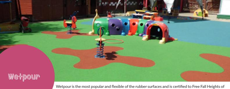
wetpour is the most popular and flexible of the rubber surfaces and is certified to Free Fall Heights of up to 3.0m. Manufactured from SBR rubber sub base with EPDM topping to create a hard wearing top surface, our wet pour can be used in all play environments. Available in a wide range of colours, including black, red, blue, green and yellow. We can create patterns or patches of different colours to suit your site.
