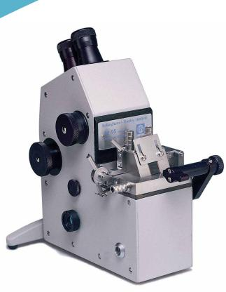
More stringent requirements of quality control and, in some cases, legislation, mean that greater accuracy is being demanded of refractometers. The Abbe 60 Direct Reading models, available in two measuring ranges, have been designed to meet these requirements.
