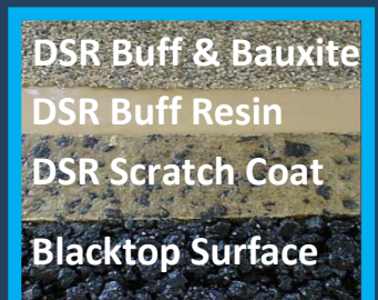
Fig 24: Scratch Coat Build-Up
