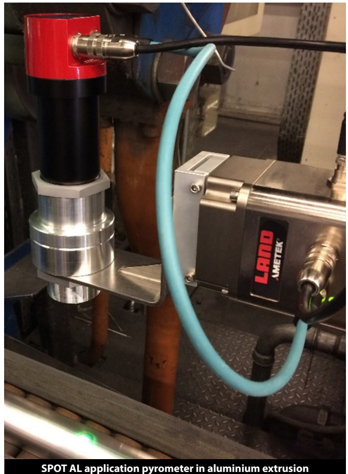
SPOT AL application pyrometer in aluminium extrusion
