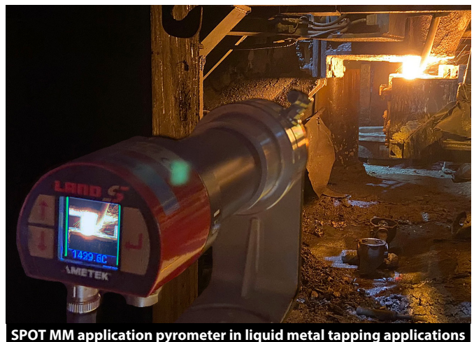
SPOT MM application pyrometer in liquid metal tapping applications
