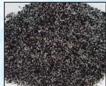
Granular Activated Carbon (GAC)
