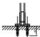
stainless steel supporting leg with flat stainless steel cover sleeve or aluminium with flat aluminium cover sleeve
