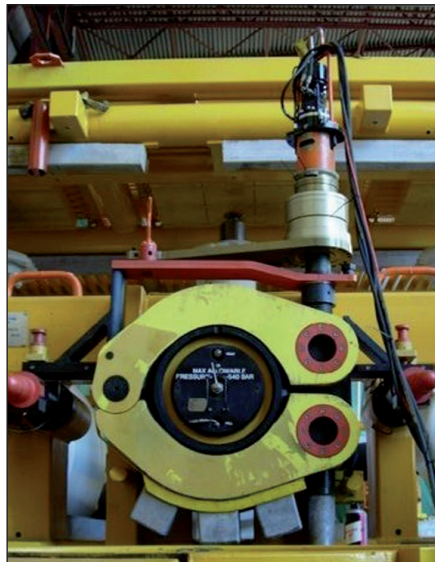
Torque multiplier specifically for actuating wet pipe connector clamps requiring torque of up to 63,000Nm.
