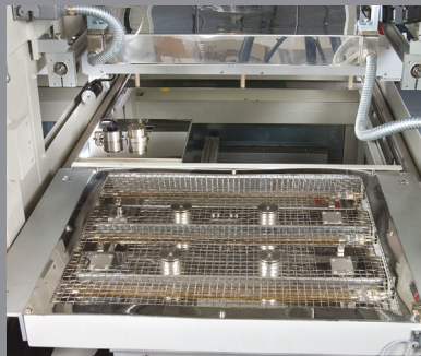
BOTTOM SIDE SLIDE IN/OUT IR PRE-HEAT
